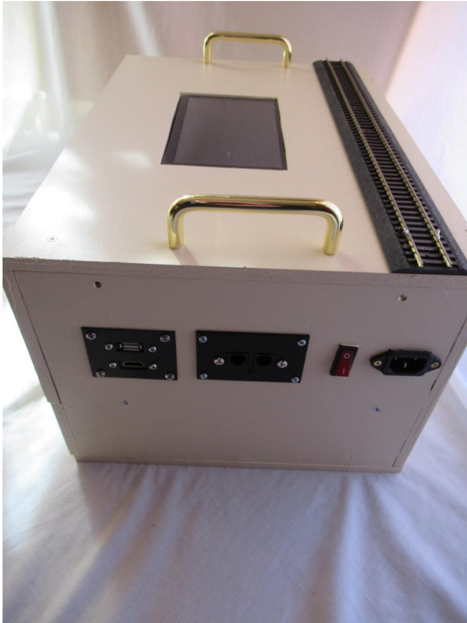
Figure 5: The connections - HDMI and USB on the left, PCP in the middle
