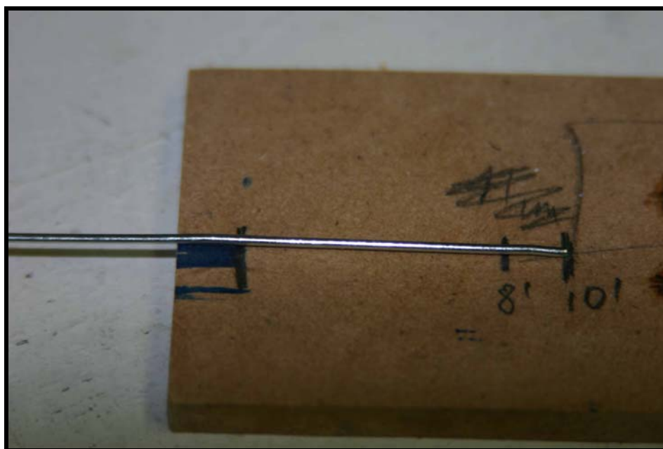
Figure 2. Cutting jig for fence posts.
