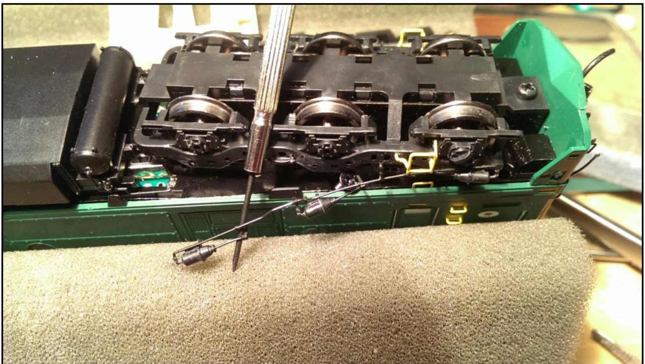
Figure 1. Cylinders removed to expose unnecessary screw. One of the light switches for number lights can also be seen to the left.
