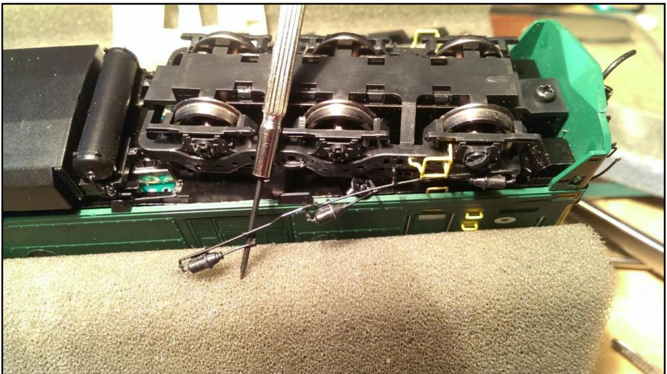
Figure 1. Cylinders removed to expose unnecessary screw. One of the light switches for number lights can also be seen to the left.
